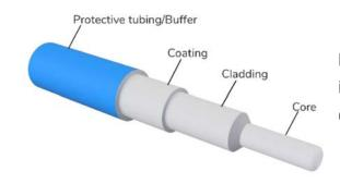
Excalibur fibers employ four separate layers of material including a glass core, glass cladding, coating and protective outer tubing, also referred to as the buffer layer.
