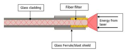
The Excalibur fiber inhibits stray energy from entering the cladding layer, preventing thermal damage to the fiber and ureteroscope. An additional glass ferrule serves as a blast shield, preventing energy from damaging the laser's optics.
