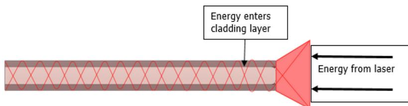
Without a filter, laser energy can easily enter the cladding layer of the fiber. If the fiber is deflected and there is too much energy in the cladding layer, the energy can spill into the coating layer resulting in major thermal damage to the fiber and flexible ureteroscope.
