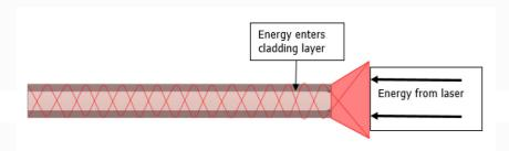
Without a filter, laser energy can easily enter the cladding layer of the fiber. If the fiber is deflected and there is too much energy in the cladding layer, the energy can spill into the coating layer resulting in major thermal damage to the fiber and flexible ureteroscope.
