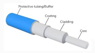
Excalibur fibers employ four separate layers of material including a glass core, glass cladding, coating and protective outer tubing, also referred to as the buffer layer.
