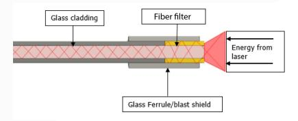
The Excalibur fiber inhibits stray energy from entering the cladding layer, preventing thermal damage to the fiber and ureteroscope. An additional glass ferrule serves as a blast shield, preventing energy from damaging the laser's optics.
